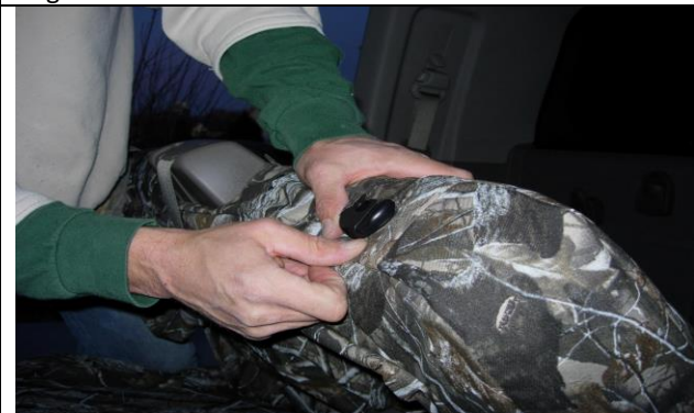
Step 11. Driver & Passenger Top/DT&PT: Tuck the fabric under the plastic for the headrests.
