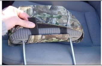
**Step 14. Headrests/H:** Slide the cover on with the extending hook Velcro<sup>™</sup> to the front, connecting them to the loop Velcro<sup>™</sup> as shown.
