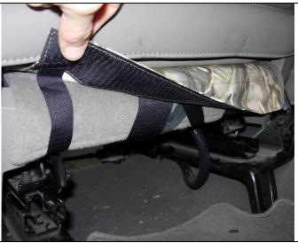
**Step 4. Driver & Passenger Bottoms/DB&PB:** From the back of the seat, pull back on the cover and press the hook Velcro<sup>™</sup> to the carpet as shown.
