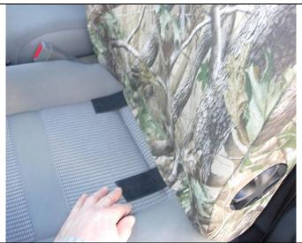
**Step 6. Driver & Passenger Tops/DT&PT:** Tuck the Velcro<sup>™</sup> into the seat. Line up the seams of the seat cover to the seams of your seat, they should closely match. Gently pull on the hook Velcro<sup>™</sup> with one hand from the back while sliding your other hand down the front of the seat cover in a smoothing action, pin the Velcro<sup>™</sup> to the seat with the front hand, then press the Velcro<sup>™</sup> together with the other hand in back.
