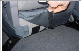
**Step 13. Middle Bottom/MB:** Pull the cover back and press it to the carpet as shown. Put the seatbelts through the elastic sewn to the seat cover.
