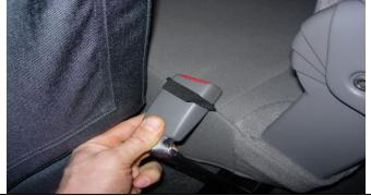
**Step 11. Middle Bottom/MB:** Temporarily remove the seatbelt from its elastic restraint.
