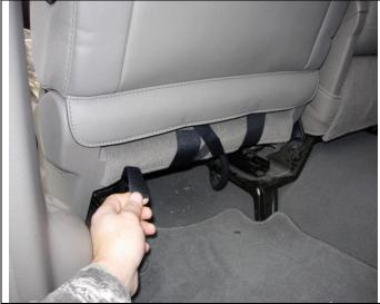
Step 1. Driver & Passenger Bottoms/DB&PB: All of the parts of your seat cover are labeled on the inside. Use the "Seat Cover Piece Identification Chart" to identify the pieces. Place the seat cover on with the long hook (sticky) Velcro™ to the front. Line up the seams of the seat cover to the seams of the seat, they should closely match. Route the hook Velcro™ under the front of the seat, avoiding any seat mechanisms, and press them to the carpet on the back edge as shown.
