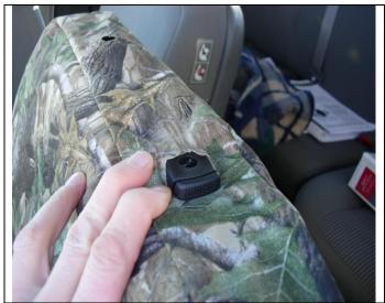
**Step 5. Driver & Passenger Tops/DT&PT:** Temporarily remove the headrests by depressing the push button release and gently lifting up. Slide the seat cover on with the extending hook Velcro<sup>™</sup> to the front. Tuck the seat cover under the plastic for the headrest starting with the push button release.
