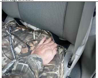
**Step 3. Driver & Passenger Bottoms/DB&PB:** Tilt the back rest forward and tuck the back edge of the seat cover into the seat.
