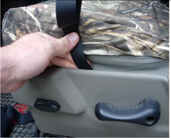
**Step 2. Driver & Passenger Bottoms/DB&PB:** Slide the outside edge hook Velcro<sup>™</sup> down between the plastic cowling and the seat. Look under the front of seat to locate it, and then route it at an angle, avoiding mechanisms, and press it to the carpet on the back edge. The inside edge hook Velcro<sup>™</sup> connects similarly at an angle to the carpet on the back edge of the seat bottom.
