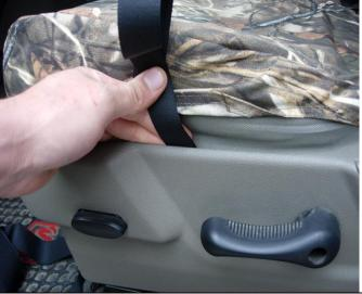
**Step 2. Driver & Passenger Bottoms/DB&PB:** Next, tuck the back edge of the seat cover into the seat, pull back, and press the hook Velcro<sup>™</sup> to the loop Velcro<sup>™</sup> sewn on the back of the seat cover. Connect the plastic buckles under the back of the seat to the rear foam support wire, then back to the loop Velcro<sup>™</sup> on the back edge of the seat cover, trim the excess.
