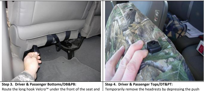
Route the long hook Velcro<sup>™</sup> under the front of the seat and stick them to the loop Velcro<sup>™</sup> sewn on the back edge of the seat cover. Make sure the Velcro is routed above any wires or bars.
