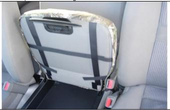
**Step 12. Middle Bottom/MB:** Mate the fasteners to the carpet on the bottom of the seat and the long side to side fasteners to each other.
