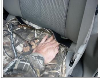
**Step 1. Driver & Passenger Bottoms/DB&PB:** All of the parts of your seat cover are labeled on the inside. Use the "Seat Cover Piece Identification Chart" to identify the pieces. Place the seat cover on with the long hook (sticky) fasteners to the front. Line up the seams of the seat cover to the seams of the seat, they should closely match. Tuck in the back edge of the seat cover and tilt the back rest forward.
