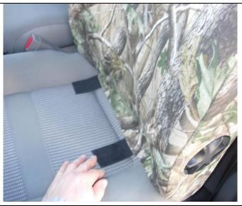
Step 6. Driver and Passenger Tops/DT&PT: Tuck the hook Velcro<sup>™</sup> into the seat. Line up the seams of the seat cover to the seams of your seat, they should closely match. Gently pull on the hook Velcro<sup>™</sup> from the backside with one hand while sliding your other hand down the front of the seat cover taking up the slack in the seat cover. Push the front hand thru to the back pinning the Velcro<sup>™</sup> to the seat, then connect the Velcro<sup>™</sup> for a snug fit.
