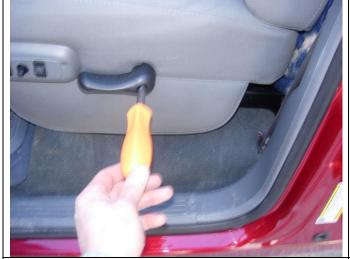
**Step 1. Driver and Passenger Bottoms/DB&PB:** The parts of the seat cover are labeled inside. Use the "Seat Cover Piece Identification Chart" to identify the parts. Temporarily remove the screw from the recline lever using a Phillips screwdriver.
