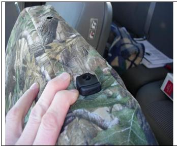
**Step 5. Driver and Passenger Tops/DT&PT:** Temporarily remove the headrests by depressing the push button release and gently lifting up. Slide the seat cover on with the extending hook Velcro<sup>™</sup> to the front. Tuck the seat cover under the plastic for the headrest starting with the push button release.
