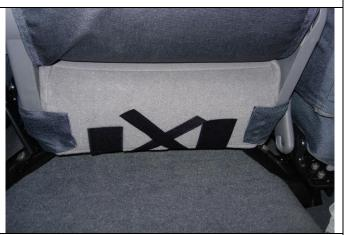
**Step 12. Middle Bottom/MB:** Pull the left and right sides of the seat cover around to the back and press them to the Loop Velcro<sup>™</sup> sewn on the back edge(not shown). Route the long hook Velcro<sup>™</sup> under the front of the seat and connect them to the loop Velcro<sup>™</sup>. Route the long side hook Velcro<sup>™</sup> under the seat and connect them at an angle forming an "X" in the middle as shown.
