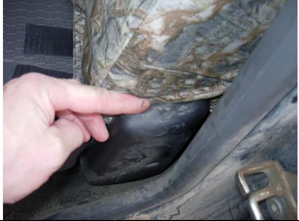
Step 6. Driver and Passenger Top/DT&PT: Pull down the left and right side of the covers and tuck the cover behind the plastic on the outside edge.
