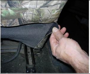
2. Driver & Passenger Bottom/DB&PB: Line up the hole for the recline lever and put it back on the seat. Tuck in the back edge of the seat cover in a little just to hold the seat cover in place. Line up the seams of the seat cover to the seams on the seat, they should match closely. Pull the material behind the lever around to the back and press the hook Velcro<sup>™</sup> onto the carpet fuzz on the back edge of the seat.
