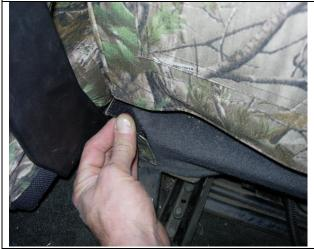
3. Driver & Passenger Bottom/DB&PB: Continue to line up the seams of the seat cover to the seams of the seat. Slide your hand around the sides of the seat cover from the outside edge to the front, then along the inside edge by the seat belt, taking up the slack, then press the hook Velcro<sup>™</sup> onto the back edge as shown.
