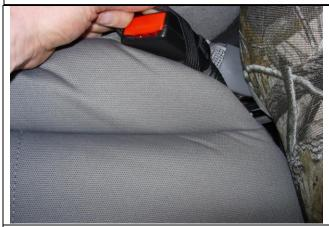
**Step 1. Driver & Passenger Bottoms/DB&PB:** Remove the seatbelt from its factory elastic on the insides of both seats. All the parts of the seat cover are labeled inside. Use the Seat Cover Part Identification Chart to ID parts. All the parts are labeled on the inside right corners of the seat cover.
