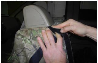
**Step 9.** Driver & Passenger Tops/DT&PT: Tuck the fabric under the plastic and connect the Velcro<sup>™</sup> behind the plastic seat belt housing.
