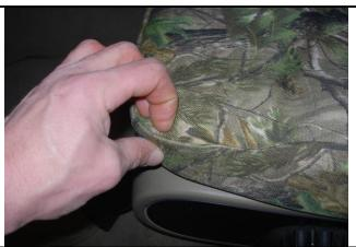
Step 2. Driver & Passenger Bottoms/DB&PB: Place the seat cover on with the long hook Velcro<sup>™</sup> to the front and tuck the back edge of the cover into the seat. Line up the seams of the seat cover to the seams of the seat, they should closely match. Work the material inside the seat cover outward, or from fingers to thumb.
