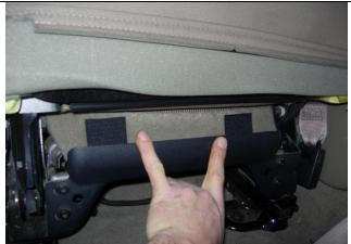
**Step 3.** Driver & Passenger Bottoms/DB&PB: Route the long hook Velcro<sup>™</sup> under the seat avoiding any seat mechanisms, in front of the metal bar, and press them to the carpet on the back edge of the seat.
