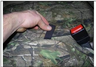
**Step 5.** Driver & Passenger Bottoms/DB&PB: Tuck the long inside edge hook Velcro<sup>™</sup> down next to the middle bottom and route it through the gap between the seat and seat slide and mate it to the carpet on the back edge. If it sticks to carpet on the inside edge of the seat, pull it back up and cut the Velcro<sup>™</sup> down to 4" and press it to the carpet on the side of the seat.
