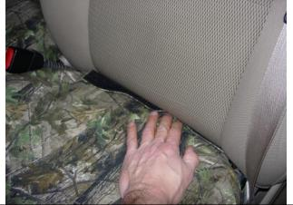
**Step 6.** Driver & Passenger Bottoms/DB&PB: Tuck the back edge of the seat cover into the seat. Pull back hard on the fabric of the seat cover and press it to the carpet on the seat working from one side to the other. You may have to re-adjust the front, left and right side, and back Velcro<sup>™</sup> for the best fit.
