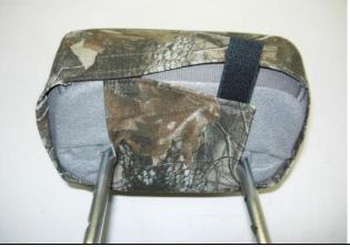
**Step 16.** Headrests/H: Connect the Velcro<sup>™</sup> in back as shown.
