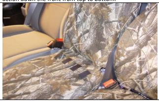
**Step 13.** Armrest/A: Place the armrest cover on with the hook Velcro<sup>™</sup> to the front. As in Step 2, line up the seams of the armrest cover to the seams of the armrest.
