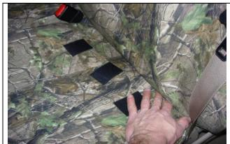
**Step 11. Driver & Passenger Tops/DT&PT:** Again, line up the seams as in Step 2. fold the backrest forward and tuck the Velcro<sup>™</sup> into the seat and connect them to the loop Velcro<sup>™</sup> sewn inside the back edge. Do this by gently pulling on the Velcro<sup>™</sup> from behind with one hand while using your other hand in a smoothing action down the front from top to bottom.
