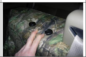
**Step 8.** Driver & Passenger Tops/DT&PT: Carefully open the seat cover bottom and side. Place the seat cover on with the hook fasteners to the front and tuck the cover between the seat belt and the seat as shown. Like Step 2, line up the seams of the seat cover to the seams of the seat.
