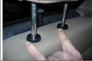
**Step 7. Driver & Passenger Tops/DT&PT:** Temporarily remove the headrests. Slide the seat forward and recline the backrest. Depress the push button releases on the plastic, and gently lift up. One release will be easily visible, the left side button is flush with the plastic and hard to see.
