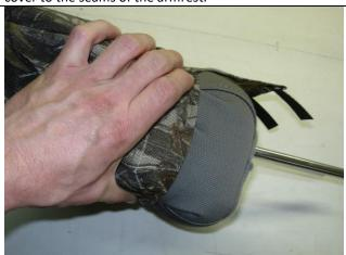
**Step 15. Headrests/H:** Slide the cover on with the hook Velcro<sup>™</sup> to the front. Notice how the headrest needs to be compressed to get the cover on. It relaxes back once the cover is pulled on.
