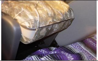
**Step 14.** Armrest/A: Move the armrest back and forth and carefully tuck the cover behind the plastic covers of the hinge area. connect the Velcro<sup>™</sup> on the back edge as shown.
