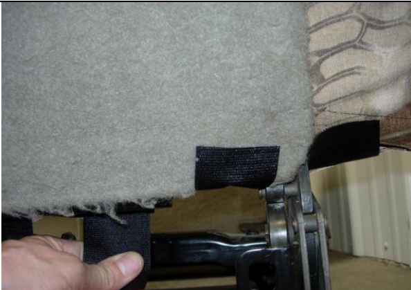
Step 15. Driver & Passenger Tops/DT&PT: Using one hand in a smoothing action down the front of the seat while gently pulling on the front hook Velcro™, then press it to the fuzz on the Cargo Flap as shown.
