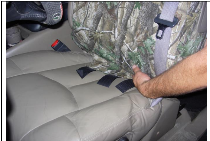
Step 7. Driver and Passenger Tops: Tuck the long hook Velcro™ into the seat.
