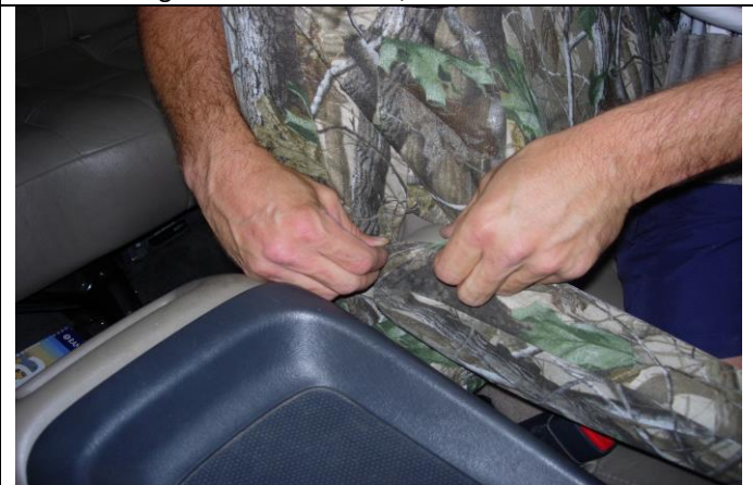
Step 10. Driver and Passenger Armrests: Connect the Velcro™ behind the armrest. This will also be a difficult maneuver because it is so snug and there isn't much room behind the armrest.
