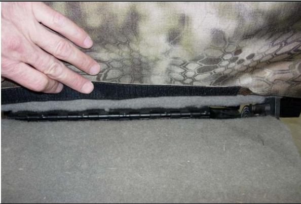
Step 13. Driver & Passenger Tops/DT&PT: Press the back edge Hook Velcro™ to the fuzz just about the hinge on the backside of the seat.
