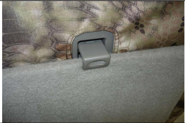
Step 14. Driver & Passenger Tops/DT&PT: Line up the hole provided for the latch. Latch the cargo flap to the backside of the seat.
