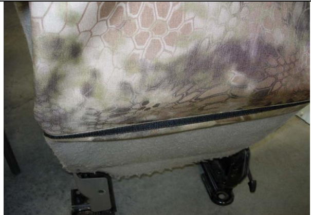
Step 16. Driver & Passenger Cargo Flaps/DCF&PCF: Turn the cover inside out so the hook Velcro™ doesn't stick to the carpet fuz. Pull all the way down and press the hook Velcro™ to the carpet fuz next to the hinge.
