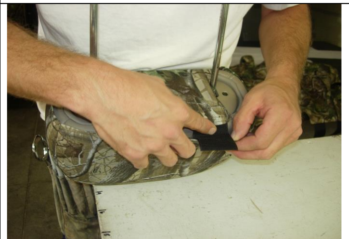
Step 12. Headrests: Tuck the hook Velcro™ inside the back edge and press them to the loop Velcro™ sewn under the back edge.
