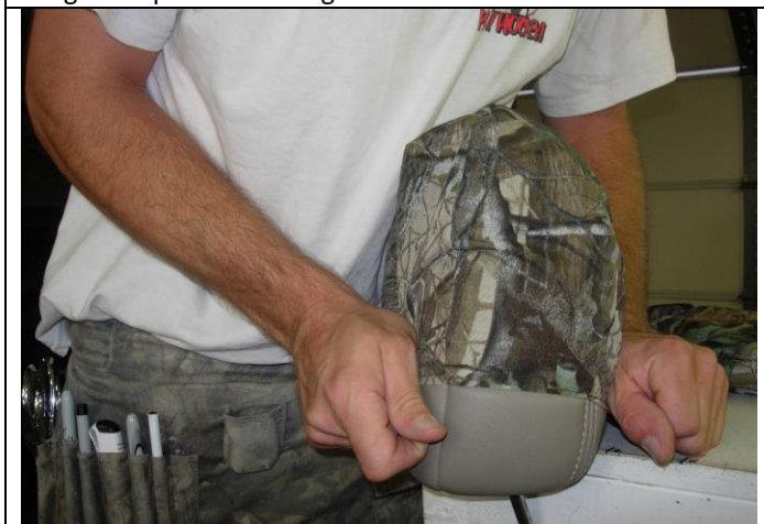
Step 11. Headrests/H: Compress the headrest and slide the covers on with the hook Velcro™ to front. Use the corner of a table, or do it with the headrest still in the seat.
