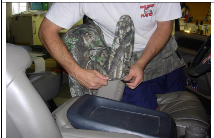
Step 9. Driver and Passenger Armrests/DA & PA: Slide the armrest cover on with the cut out for the hinge bolt on the inside. This will be difficult as they are sewn to fit very snug to help avoid shifting.
