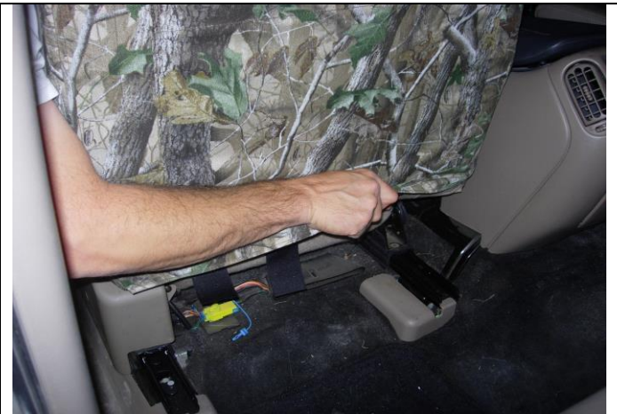
Step 8. Driver and Passenger Tops: Gently pull the Velcro™ from behind the seat with one hand and use your other hand in a smoothing motion from top to bottom to tighten the seat cover, then connect the Velcro™.
