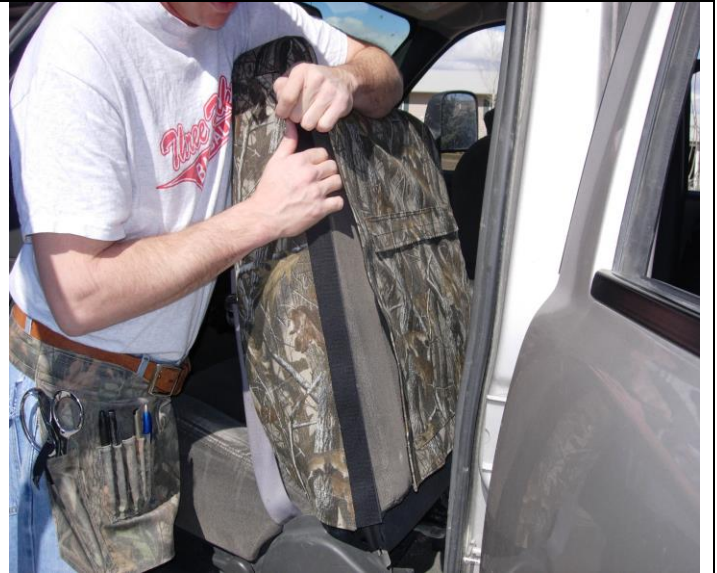
Step 14. Driver and Passenger Tops: Next, start at the top, line up the seams, and connect the Velcro™.
