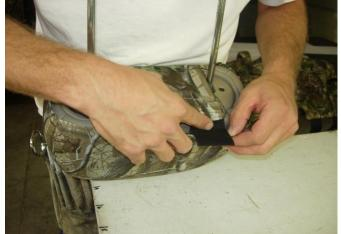
**Step 12. Headrests:** Tuck the hook Velcro<sup>™</sup> inside the back edge and press them to the loop Velcro<sup>™</sup> sewn under the back edge.
