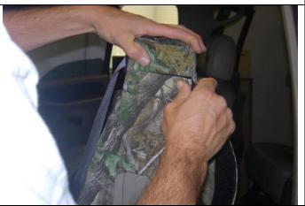
**Step 4. Driver and Passenger Tops:** Seats with Side Impact Airbags, tuck the fabric of the seat cover behind the rubberized rectangular airbag cover on the outside edge of the Driver & Passenger shown in Step 5. Connect the horizontal Velcro<sup>™</sup> as shown.
