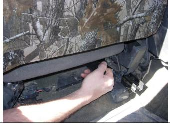
**Step 17. Driver and Passenger Bottoms:** If you have electric seats be sure to lift the seat up as high as it will go. This will pull everything away from your seat and free up some space. With the seat cover pulled back into position, route the long hook Velcro<sup>™</sup> under the seat, avoiding any seat mechanisms, and press them to the carpet located on the back edge of the seat.
