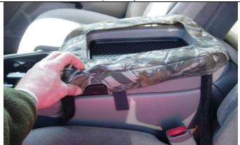
**Step 21. Lid/L:** Place the lid cover on with the cut-out for the push button release on the front left side (thumb).
