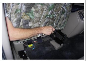
**Step 8. Driver and Passenger Tops:** Gently pull the Velcro<sup>™</sup> from behind the seat with one hand and use your other hand in a smoothing motion from top to bottom to tighten the seat cover, then connect the Velcro<sup>™</sup>.
