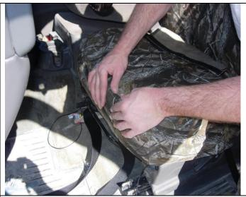
**Step 16. Driver and Passenger Bottoms:** Use your thumbs to work the seat cover fabrics on the inside of the cover, out. Try to match the seams of the seat cover to the seams of your seat for the best possible fit.
