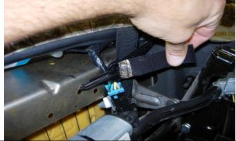
**Step 19. Driver and Passenger Bottoms:** View of under the front of the driver's seat. Push the plastic hook into the oblong hole, pull it tight, and mate the Velcro<sup>™</sup>. If no hole exists, see step 20.
