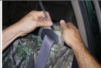
**Step 3. Driver and Passenger Tops:** Carefully tuck the fabric of the seat cover behind the plastic for the seat belt using something thin like a feeler gauge or screwdriver.
