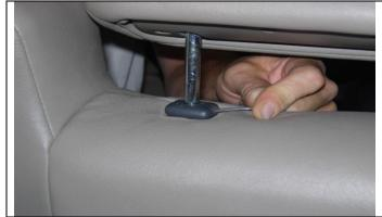
**Step 1. Driver and Passenger Tops/DT & PT:** Temporarily remove the headrests by lifting it up all the way and inserting a heavy paper clip into the holes in the plastic as shown. Do this one at a time, gently lifting up and holding pressure until the headrest releases. The pieces of the seat cover are labeled inside. Use the "Seat Cover Piece Identification Chart" to identify the pieces of the seat cover.
