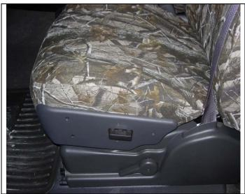
**Step 15. Driver and Passenger Bottoms/DB & PB:** Place the seat cover bottoms on with the long hook Velcro<sup>™</sup> to the front. For vehicles with electric seat controls, tuck the cover behind the plastic cowling starting in back, then do the front. It should like the picture once in place.
