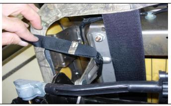
**Step 20. Driver and Passenger Bottoms:** View of under the front of the driver's seat. Push the plastic hook over the seat brace as shown, pull it tight, connect the Velcro<sup>™</sup>, and trim off the excess with a scissor.
