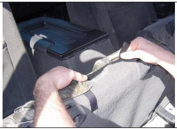
**Step 13. Drivers Bottom/DB:** Press the hook Velcro<sup>™</sup> sewn inside the cover to the carpet in the recession for the seatbelts as shown (left thumb).
