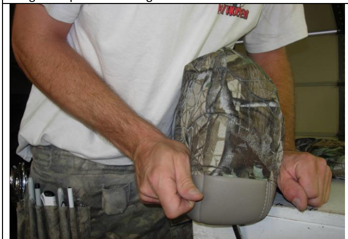
Step 11. Headrests/H: Compress the headrest and slide the covers on with the hook Velcro™ to front. Use the corner of a table, or do it with the headrest still in the seat.
