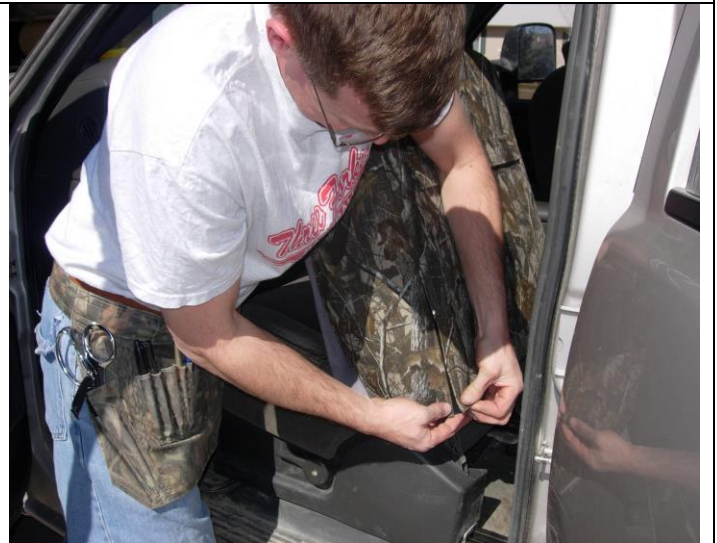
Step 16. Driver and Passenger Tops: Keep re-fastening the outside edge Velcro™ until the seams meet and the seat cover lines up at the bottom.
