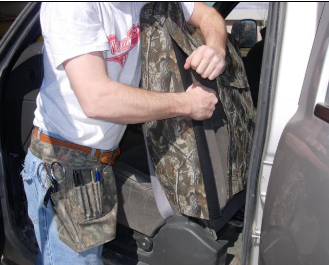
Step 15. Driver and Passenger Tops: Working from the top, fasten the Velcro™ a few inches at a time, using what I call a "bear hug" method" with some downward pressure.
