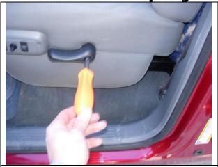
Step 1. Driver and Passenger Bottoms DB/PB: Use the "Seat Cover Piece Identification Chart" to indentify the different parts of the seat cover. Temporarily remove the recline lever using a Phillips screwdriver.
