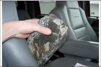
**Step 13. Armrests/DA&PA:** Open the armrests in back and slide them all the way on, lining up the seams of the cover to the seams of the armrest.
