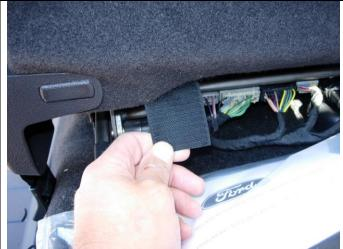
**Step 7. Driver & Passenger Bottoms/DB&PB:** Route the long front hook fasteners under the front of the seat, avoiding seat mechanisms, and mate them to the carpet on the back edge of the seat bottom.
