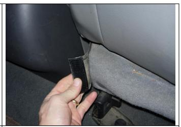
**Step 6. Driver & Passenger Bottoms/DB&PB:** View from behind the passenger side. Pull back hard on the inside edge part of the seat cover (shown) and route it around to the back, connecting it to the carpet on the back edge of the seat.
