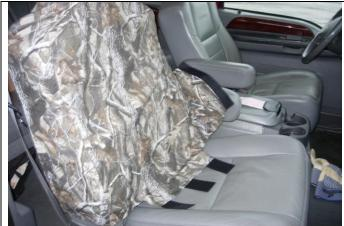
**Step 9. Driver & Passenger Top/DT&PT:** Carefully open the seat cover and slide it on with the extending hook Velcro<sup>™</sup> to the front and the cut-out for the armrest to the inside. Move the armrest up and down while tucking the fabric behind it.
