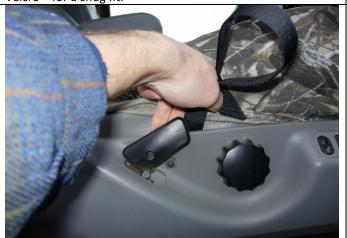
**Step 3. Driver & Passenger Bottoms/DB&PB:** Optional but helpful: Temporarily removing the Phillips screw in the plastic cowling below the recline lever (shown) will make the routing of the outside edge hook strap between the seat and the plastic easier. Put the screw back in after completing step 4.
