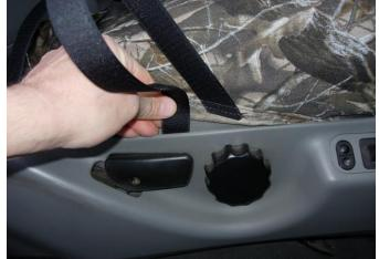
**Step 4. Driver & Passenger Bottoms/DB&PB:** For vehicles with electric controls: Use the controls to lift the seat up all the way, giving yourself more clearance. Slide the long outside edge hook Velcro<sup>™</sup> between the seat and plastic cowling, mating it at an angle to the carpet on the back edge of the seat.
