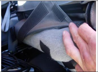
**Step 8. Driver & Passenger Bottoms/DB&PB:** Lastly, pull back hard on the rear part of the seat cover, center it, and connect it to the carpet on the back edge of the seat by pressing it hard into the carpet on the seat bottom.
