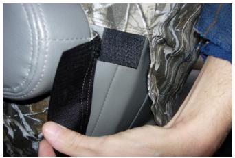
**Step 10. Driver & Passenger Top/DT&PT:** Mate the Velcro<sup>™</sup> directly behind the armrest.
