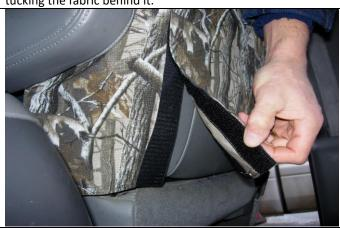
**Step 11. Driver & Passenger Top/DT&PT:** Next, mate the vertical Velcro<sup>™</sup> starting at the top, working your way down a few inched at a time.
