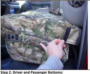
Slide the seat cover over the upholstered flap on the outside, then position the hole for the recline lever and put it back on. Note: Your style of seat does NOT have electric controls like the picture shows.
