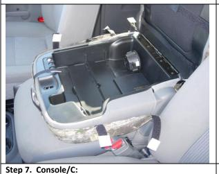
With the console in the up position, slide the console cover on and tuck it in on the bottom. Fold the console down, holding it in position with one hand. Pull the cover up to cover the material of the console. Note where the Velcro™ will lay inside the cavity. Fasten the right side and left side rear hook Velcro™ to
