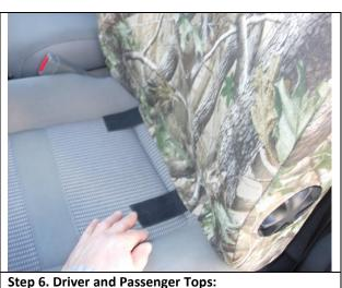
Tuck the hook Velcro™ into the seat. Line up the seams of the seat cover to the seams of your seat, they should closely match. Gently pull on the hook Velcro™ with one hand from behind the seat while sliding your other hand down the front of the seat cover taking up the slack in the seat cover. Lastly, connect the hook Velcro™ to the loop Velcro™ sewn inside the back edge.
