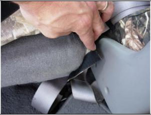
**Step 16. Driver & Passenger Bottom/DB&PB:**Pull the inside edge piece of material around to the back and mate it to the carpet on the seat as shown.
