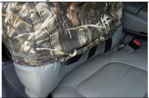
Step 6. Driver & Passenger Top/DT&PT: Slide the seat cover tops on with the extending hook  $Velcro^{TM}$  to the front.
