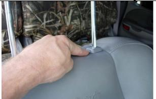
**Step 1.**Recline the backrests and temporarily remove the headrests by depressing the push button release and gently lifting up.
