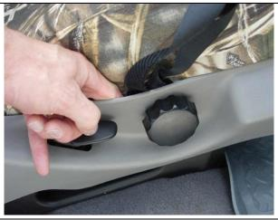
Step 14. Driver & Passenger Bottom/DB&PB: Use your finger to pry the plastic away from the seat, and stuff the side Velcro™ in between the seat and plastic.
