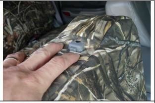
**Step 7. Driver & Passenger Top/DT&PT:**Tuck the seat cover under the plastic for the headrests, starting on the push button side first.
