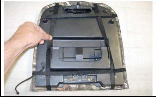
**Step 18. Lid/L:** Connect the Velcro under the lid as shown.
