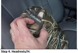
Line up the seams of the seat cover to the seams of you headrests, they should match closely. Manipulate the seat cover material outward on the left and right side from forefinger to thumb.
