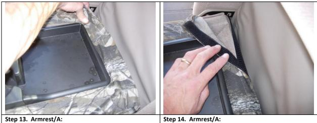
Tuck the cover behind the back of the plastic tray one corner at a time,
