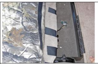
**Step 8. Driver & Passenger Top/DT&PT:** Use one hand in a smoothing action down the front of the seats while pulling on the hook Velcro<sup>™</sup> from the back, pressing them to the fuzzy carpet on the seat.
