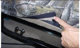
**Step 5. Driver Top/DT:** Connect the Velcro<sup>™</sup> under the left side of the armrest, then press the hook Velcro<sup>™</sup> to the fuzzy carpet at the bottom.
