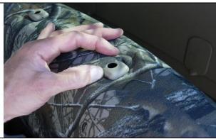
**Step 3. Driver & Passenger Top/DT&PT:** Tuck the fabric under the plastic for the headrests. Next, line up the seams of the seat cover to the seams of the seat, they should match closely.
