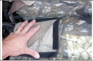
**Step 7. Passenger Top/PT:** Connect the Velcro<sup>™</sup> on the inside back edge of the passenger seat with the seat folded down.
