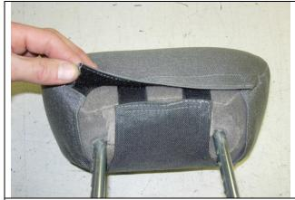
**Step 19. Headrests:** Connect the small side Velcro<sup>™</sup> first, and then connect the front hook Velcro<sup>™</sup>.
