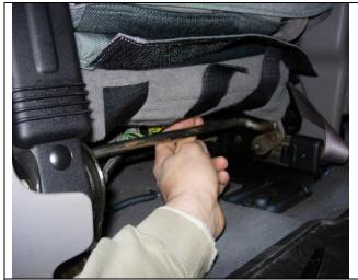
**Step 11. Driver and Passenger Bottoms/DB &PB:** Route the long hook Velcro<sup>™</sup> under the front of the seat and connect them to the carpet on the back edge of the seat. For seats with electric controls, lift the seat up. Be sure to route the Velcro<sup>™</sup> between the seat and the moving metal framework (shown) allowing the seat to move freely. Use caution reaching under the seat to avoid sharp metal edges.
