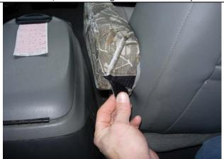
**Step 23. Driver and Passenger Armrest/DA&PA:** Connect the Velcro<sup>™</sup> behind the armrest.
