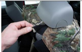
**Step 4. Driver and Passenger Top/DT & PT:s:** Connect the Velcro<sup>™</sup> behind the plastic seatbelt box on top of the seat.
