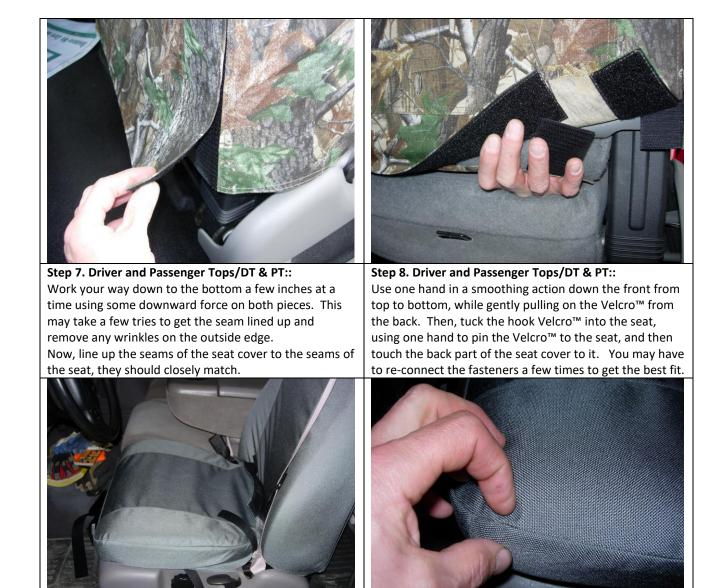
Step 9. Driver and Passenger Bottoms/DB &PB: Place the seat covers on with the long hook Velcro™ to the front. Tuck the back edge of the seat cover in behind the plastic cowling.
