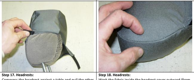
Step 17. Headrests:Step 18. Headrests:Compress the headrest against a table and pull the other<br/>side down. The headrest will spring back into shape<br/>once the headrest cover is in position.Work the fabric inside the headrest cover outward (from<br/>forefinger to thumb).
