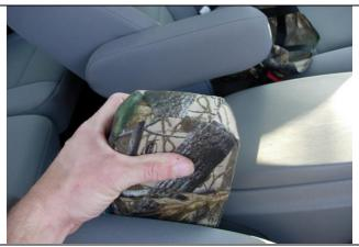
**Step 22. Driver and Passenger Armrest/DA&PA:** Recline the seats and slide the cover on with the opening towards the seat, pull it all the way down forming it to the front of the armrest with both hands.
