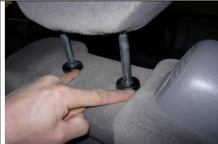
Step 1. Driver and Passenger Tops/DT & PT: Temporarily remove the headrests by lifting them up all the way. Then with slight upward pressure, simultaneously depress the two push button releases until the headrest comes out. One push button release is easily seen (pointer finger), and one is slightly hidden (pinkie).
