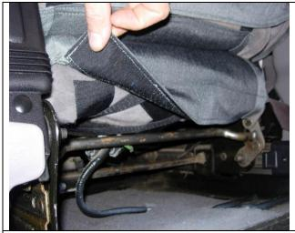
**Step 15. Driver and Passenger Bottoms/DB &PB:** Lastly, pull on the back edge of the seat cover with one hand and use the other hand in a smoothing action from front to back, taking up the slack in the seat cover, and then press the Velcro<sup>™</sup> to the carpet on the back edge of the seat.
