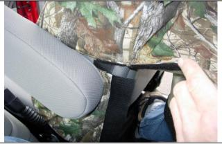
**Step 5. Driver and Passenger Tops/DT & PT::** Connect the Velcro<sup>™</sup> behind the armrest, and down the inside.
