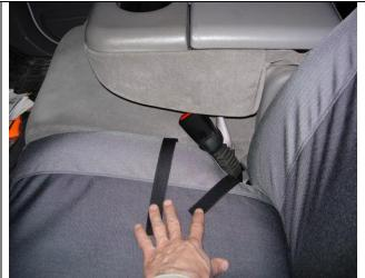
**Step 12. Driver and Passenger Bottoms/DB &PB:** Tuck the two long inside edge hook Velcro<sup>™</sup> down and under the seat. Route them carefully to the back edge of the seat and press them to the carpet on the seat. Some re-positioning of the Velcro<sup>™</sup> may be needed for the best fit.
