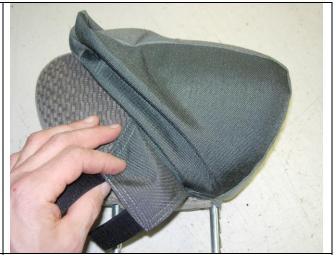
**Step 16. Headrests/H:** Open the headrest cover and slide it on one side with the extending hook Velcro<sup>™</sup> to the front. Form it to the corner as close as you can. The seams of the cover should closely match the seams of your headrest.
