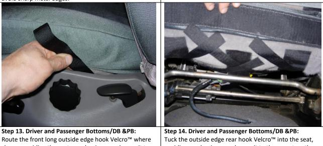
Route the front long outside edge hook Velcro<sup>TM</sup> where shown, avoiding the seats mechanisms, and press it to the carpet on the back edge of the seat. See step 14 for proper Velcro<sup>TM</sup> positions.
