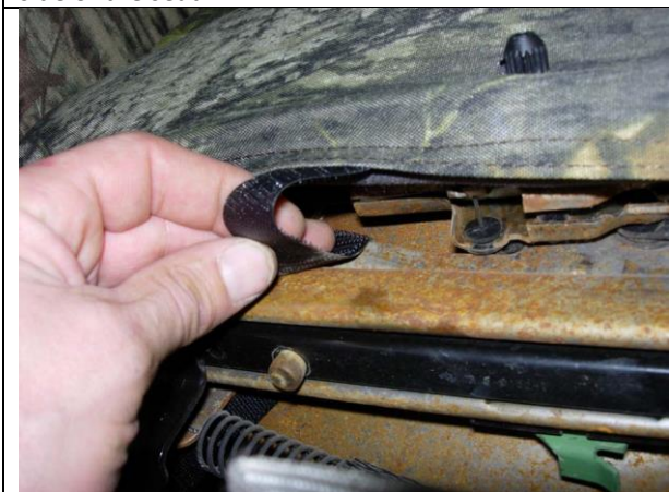
Step 13. Passenger Bottom/PB: Slide the side hook Velcro™ over the seat slides.
