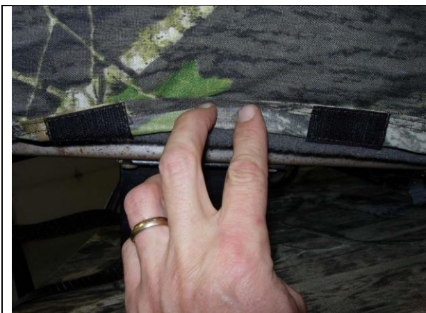
Step 11. Passenger Bottom/PB: Lift the hook Velcro™ away from the carpet on the side of the seat.
