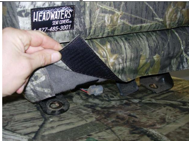
Step 16. Passenger Bottom/PB: Pull the rear most edge of the seat cover back hard and press it onto the carpet on the back edge.
