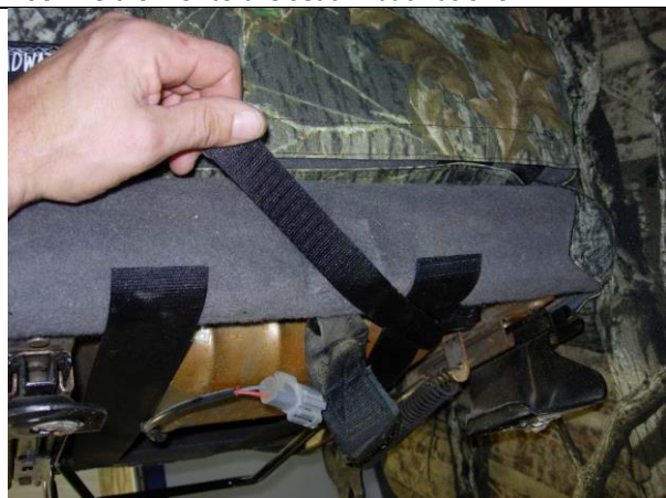
Step 14. Passenger Bottom/PB: Route them at an angle to the back edge and press them onto the carpet. Reconnect the outside edge of the seat and slide you hand along the recline lever to smooth the outside edge of the seat cover.
