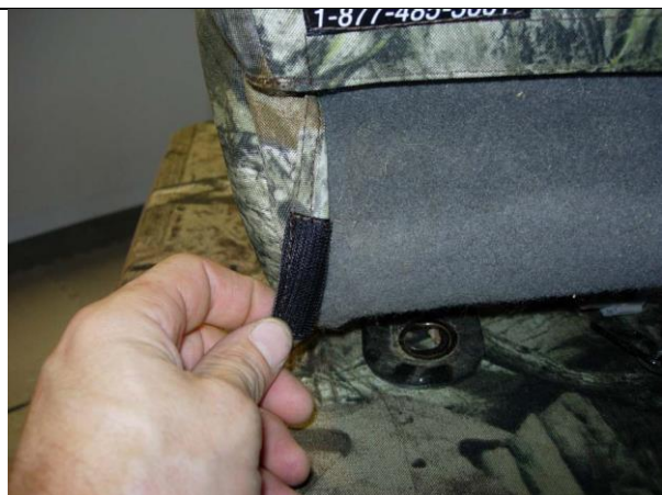
Step 12. Passenger Bottom/PB: Pull the inside around to the back hard, then press the hook Velcro™ onto the seat in back as shown.
