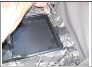
**Step 13.** Armrest/A: Tuck the cover behind the back of the plastic tray one corner at a time,
