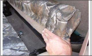
Step 9. Driver & Passenger Cargo Flap/DCF&PCF: Slide the covers on with the hook Velcro™ turned inside out, pull them all the way down and press the Velcro™ to the carpet.
