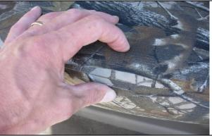
**Step 10. Driver & Passenger Bottom/DB&PB:** Find the small cut out for the seat release strap and feed the strap through it. Again, line up the seams of the seat cover to the seams on the seat. Work the fabric inside the seat cover from forefinger to thumb around the sides and front of the seat cover.
