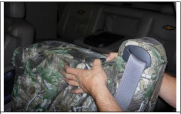
**Step 8. Driver and Passenger Tops:**Tuck the seat cover under the plastic for the headrests.
