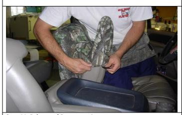
**Step 11. Driver and Passenger Armrests:**Slide the armrest cover on with the cut out for the hinge bolt on the inside. This will be difficult as they are sewn to fit very snug to help avoid shifting.
