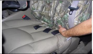
Step 9. Driver and Passenger Tops: Tuck the long hook Velcro™ into the seat.
