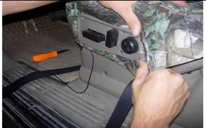
Step 16. Driver and Passenger Bottoms with elec. controls: Tuck the fabric under the back, top, and bottom of the plastic. Tighten the screws on the plastic panel. Manual seat controls: Connect the Velcro™ below the lumbar knob.
