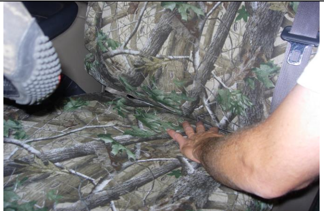
Step 18. Driver and Passenger Bottoms: Tip the back of the seat bottom down using the electric controls and tuck the back edge of the seat cover into the seat.
