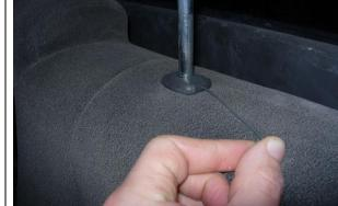
**Step 1. Driver & Passenger Top/DT&PT:** Temporarily remove the headrests by lifting them up all the way. Insert a coat hanger sized wire into the holes in the plastic, one side at a time, while holding gentle upward pressure until you feel the headrest release.
