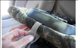
**Step 12. Armrest/A:** Slide the armrest cover on with the extending hook Velcro<sup>™</sup> to the front and the cut-out for the drink holders on top. Tuck the cover behind the front of the plastic, making sure the strap is outside the cover.
