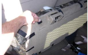
**Step 11. Driver & Passenger Bottom/DB&PB:** Press the hook Velcro<sup>™</sup> to the fuzzy carpet under the seat bottom. Do this by starting in the front and center, then working back on both sides. Then as in step 8, use one hand in smoothing action from front to back while gently pulling on the Velcro<sup>™</sup>, then pressing the hook Velcro<sup>™</sup> to the carpet.
