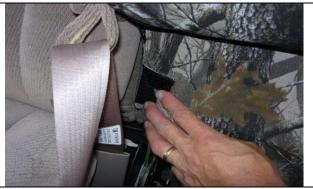
**Step 6. Driver Top/DT:** Connect the Velcro<sup>™</sup> under the right side of the armrest.
