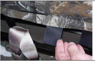
**Step 2. Driver & Passenger Top/DT:** All the parts of the seat cover are labeled inside. Use the seat cover piece identification chart to ID parts. Slide the seat covers with the extending hook (sticky) Velcro<sup>™</sup> to the front (shown).
