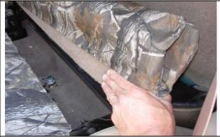
**Step 9. Driver & Passenger Cargo Flap/DCF&PCF:** Slide the covers on with the hook Velcro<sup>™</sup> turned inside out, pull them all the way down and press the Velcro<sup>™</sup> to the carpet.
