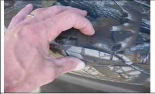
**Step 10. Driver & Passenger Bottom/DB&PB:** Find the small cut out for the seat release strap and feed the strap through it. Again, line up the seams of the seat cover to the seams on the seat. Work the fabric inside the seat cover from forefinger to thumb around the sides and front of the seat cover.
