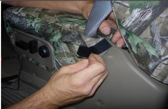
Step 17. Driver and Passenger Bottoms: Mate the Velcro™ behind the seat belt as shown.
