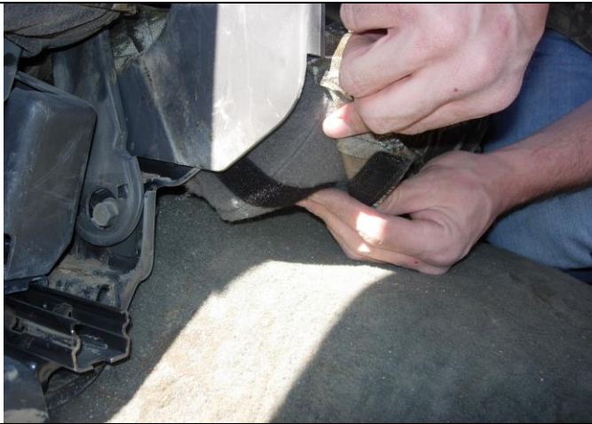
Step 13. Middle Bottom: Route the short loop Velcro™ around the back corner and connect it to the hook Velcro™ sewn inside the back edge. Work from one side to the other.
