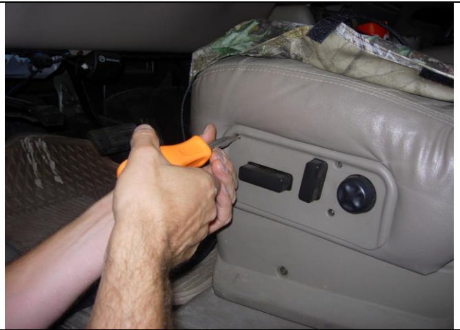
Step 14. Driver and Passenger Bottoms/DB & PB with electric seat controls: Temporarily loosen the screws on the electric control panel but don't remove them.
