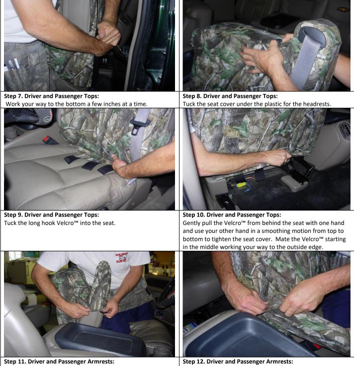
**Step 11. Driver and Passenger Armrests:** Slide the armrest cover on with the cut out for the hinge bolt on the inside. This will be difficult as they are sewn to fit very snug to help avoid shifting.
