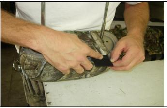
**Step 14. Headrests:** Tuck the hook Velcro<sup>™</sup> inside the back edge and connect to the loop Velcro<sup>™</sup> in back.
