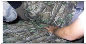
**Step 19. Driver and Passenger Bottoms:** Tip the back of the seat bottom down using the electric controls and tuck the back edge of the seat cover into the seat.
