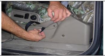
**Step 20. Driver and Passenger Bottoms:** Lift the seat all the way up (towards the roof) using the electric controls. Slide the long outside edge hook Velcro<sup>™</sup> in where shown.
