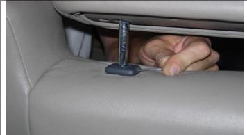
**Step 1. Driver and Passenger Tops/DT & PT:** Temporarily remove the headrests by lifting it up all the way and inserting a heavy paper clip into the holes in the plastic as shown. Do this one at a time, gently lifting up and holding pressure until the headrest releases.
