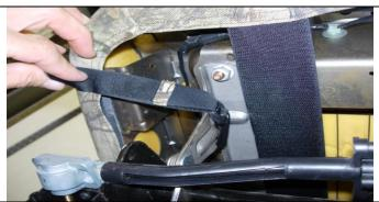
**Step 25. Driver and Passenger Bottoms:** View of under the front of the driver's seat. Push the plastic hook over the seat brace as shown.
