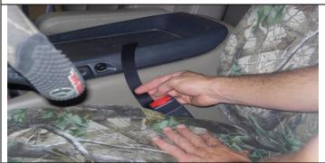
**Step 21. Driver and Passenger Bottoms:** Tuck the long inside hook Velcro<sup>™</sup> down between the console and the seat, and then lift the seat all the way up using the electric controls.
