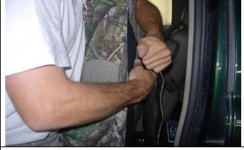
**Step 6. Driver and Passenger Tops:** Slide the seat forward, tilt the backrest ahead and connect the vertical Velcro<sup>™</sup> on the outside edge, starting at the top using the bear hug method shown.
