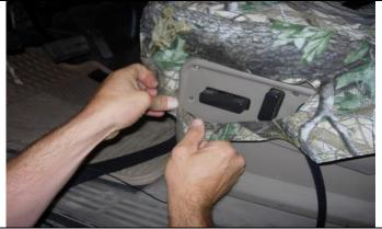
**Step 16. Driver and Passenger Bottoms:** Place the seat covers on with the long hook Velcro<sup>™</sup> to the front and the cut out for the controls on the outside edge. Tuck the fabric under the front of the plastic first.
