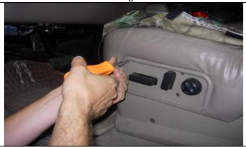
**Step 15. Driver and Passenger Bottoms/DB & PB:** Temporarily loosen the screws on the electric control panel but don't remove them.
