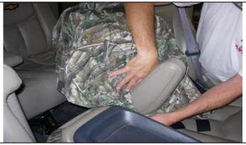
**Step 2. Driver and Passenger Tops:** All the parts of the seat cover are labeled inside. Use the seat cover piece identification chart to ID parts. Open the sides and bottom of the seat cover. Slide the seat cover over the armrest and tuck the fabric behind it.
