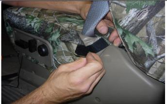
**Step 18. Driver and Passenger Bottoms:** Mate the Velcro<sup>™</sup> behind the seat belt as shown.
