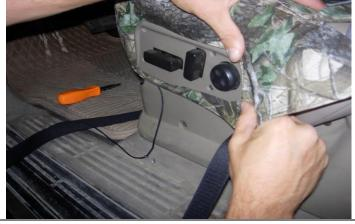
**Step 17. Driver and Passenger Bottoms:** Tuck the fabric under the back, top, and bottom of the plastic. Tighten the screws on the plastic panel.
