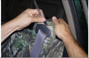
**Step 3. Driver and Passenger Tops:** Carefully tuck the fabric of the seat cover behind the plastic for the seat belt using something thin like a feeler gauge or screwdriver.
