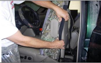
**Step 5. Driver and Passenger Tops with airbag:** Tuck the fabric behind the plastic for the side impact airbag, if the seat has an airbag.
