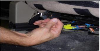
**Step 22. Driver and Passenger Bottoms:** Route the long hook Velcro<sup>™</sup> in front under the seat and connect them to the carpet on the back edge of the seat. Feel under the seat for the left and right side hook Velcro<sup>™</sup> and connect them at an angle to the carpet on the back edge of the seat.
