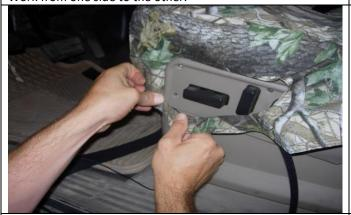
Step 15. Driver and Passenger Bottoms with elec. controls: Place the seat covers on with the long 2" wide hook Velcro™ to the front. Electric: Tuck the fabric under the front of the plastic first.
