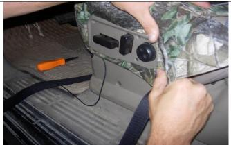
Step 16. Driver and Passenger Bottoms with elec. controls: Tuck the fabric under the back, top, and bottom of the plastic. Tighten the screws on the plastic panel.
