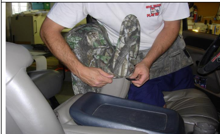
Step 11. Driver and Passenger Armrests/DA&PA: Slide the armrest cover on with the cut out for the hinge bolt on the inside. This will be difficult as they are sewn to fit very snug to help avoid shifting.
