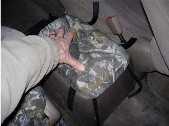
Step 23. Lid/L: Carefully separate the Velcro™ and place the lid cover on as shown with the letter "L" to the back.
