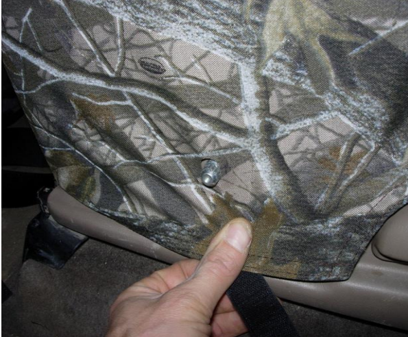
Step 11. Driver & Passenger Bottom/DB&PB: Slide the seat covers on with the long hook Velcro™ to the front. Manual controls, align the hole for the lumbar knob and push the knob back on.
