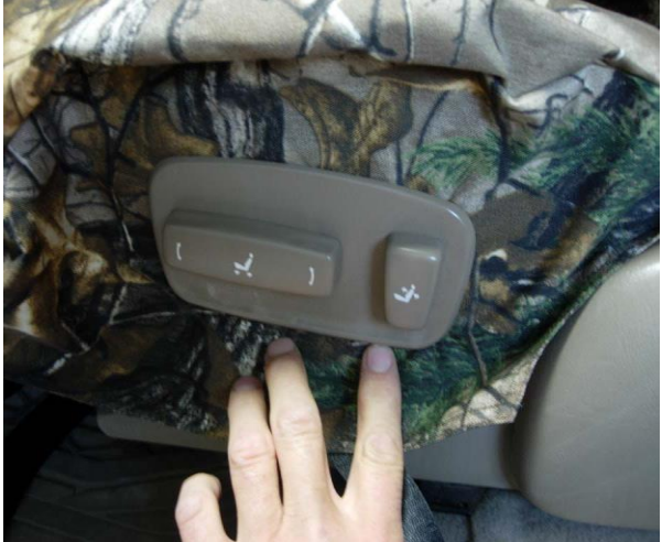
Step 12. Driver Bottom/DB: For Leather Driver seat only with electric controls. Line up the opening for the electric controls, tuck the fabric behind the plastic cowling starting on the front, then the back.
