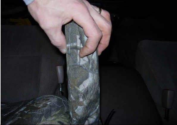
Step 19. Driver & Passenger Armrests/DA&PA: Recline the backrests and slide the armrest covers on with the cut-out to the inside.
