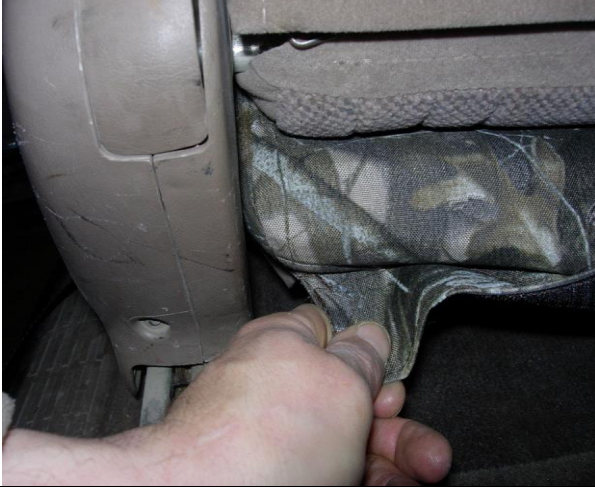
Step 13. Driver & Passenger Bottom/DB&PB: Tuck the back edge of the seat cover into the seat and pull the outside back edge around the corner as shown.
