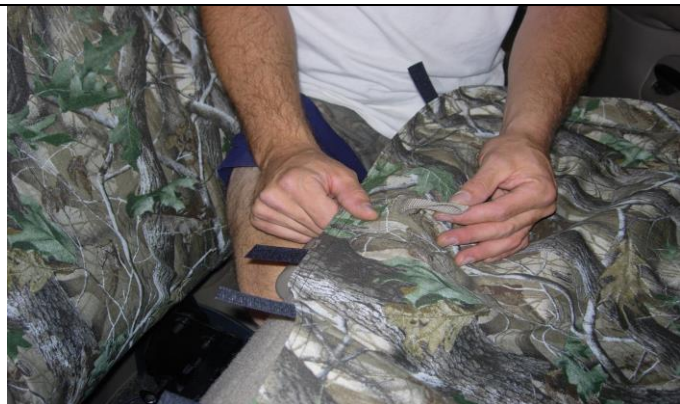
Step 12. Driver and Passenger Bottoms/DB&PB: Tilt the seat bottoms slightly forward and feed the release strap through the provided opening. Attach a few hook Velcro™ to the carpet on the seat behind the strap. Pull the seat cover over the front of the seat and mate the hook Velcro™ under the front of the seat.
