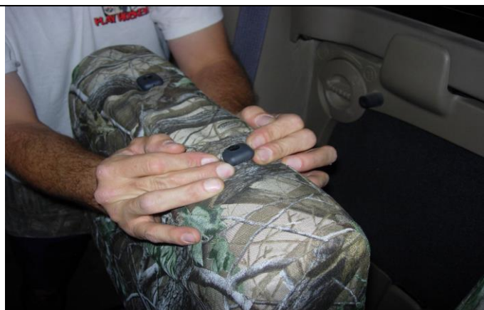
Step 8. Passenger Top/PT: Same as the driver's seat, tuck the fabric under the plastic for the headrests.
