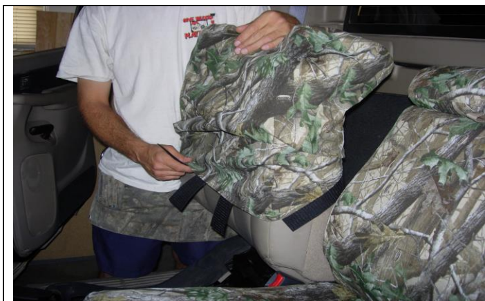
Step 7. Passenger Top/PT: Open the bottom and inside of the seat cover and slide it on with the long hook Velcro™ to the front.
