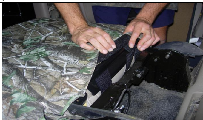
Step 10. Passenger Top/PT: Mate the hook Velcro™ to the loop Velcro™ sewn inside the back edge starting on one side moving to the other.
