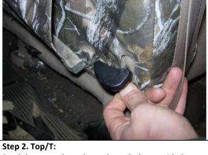
Feed the seat release lever through the provided openings on each side. Line up the seams of the seat cover to the seams of the seat, they should match closely.
