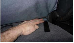
**Step 4. DT&PT/Driver & Passenger Top:** Tuck the front edge of the cover in, along with the two hook Velcro<sup>™</sup> sewn on the front edge.
