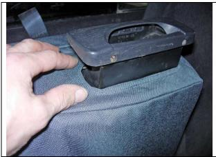
**Step 9. DB&PB/Driver & Passenger Bottom:** Lift the drink holders out of the front of the Passenger seat and work the seat cover around it.
