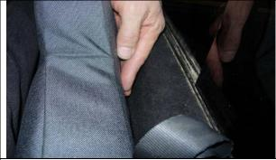
**Step 3. DT&PT/Driver & Passenger Top:** Press the hook Velcro<sup>™</sup> onto the carpet that's on the backside of the seat.
