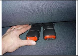
**Step 14. DB&PB/Driver & Passenger Bottom:** Lastly, slide the seatbelts thru the elastic sewn on the seat covers.
