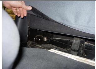
**Step 13. DB&PB/Driver & Passenger Bottom:** Pull the bottom of the cover tight and press it the carpet under the seat as shown.
