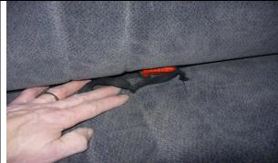
**Step 1. Prepare the seat for Installation:** Temporarily slide the seat belts out of the elastic. All parts of the seat cover are labeled on the inside right of each part. Use the Seat Cover Part ID Chart.
