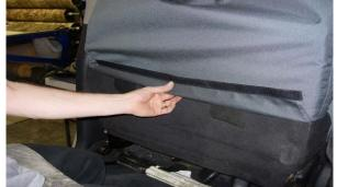
**Step 8. DB&PB/Driver & Passenger Bottom:** Slide the seat covers on keeping the Velcro<sup>™</sup> turned inside out so it doesn't stick while pulling it down.
