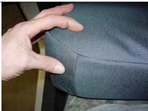
**Step 11. DB&PB/Driver & Passenger Bottom:** Pull the cover back into position, again lining the seams of the seat cover to the seams on the seat, working the material inside the cover from forefinger to thumb.
