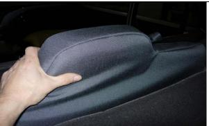
**Step 2. DT&PT/Driver & Passenger Top:** Form the top of the seat cover to the top of the seat, lining up the seams of the seat cover to the seams on the seat, they should match closely.
