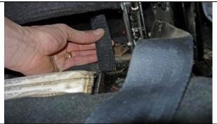
**Step 5. DT&PT/Driver & Passenger Top:** Lift the seat bottoms up, feed the two Velcro<sup>™</sup> thru.
