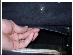
**Step 12. DB&PB/Driver & Passenger Bottom:** Pull the top edge of the seat cover tight and press the hook Velcro<sup>™</sup> to the carpet on the back edge of the seat.
