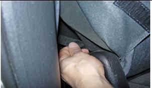
**Step 6. DT&PT/Driver & Passenger Top:** Wrap the Velcro around to the side and press them to the carpet on the side of the seat.
