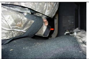
**Step 14. Middle Bottom/MB:** Route the front hook Velcro<sup>™</sup> under the seat, mating them to the carpet on back of the seat. Pull the left and right sides back and mate them to the carpet. Step 14. Middle Bottom/MB: Slide the driver and passenger seats all the way forward and place the cover on with the extending hook Velcro<sup>™</sup> to the front. Tuck the cover behind the plastic drink holders and line up the seams along the front and sides.
