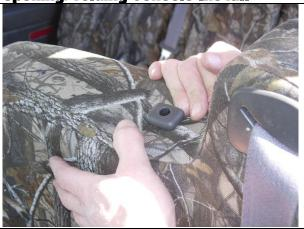
**Step 2. Driver & Passenger Tops/DT & PT** Carefully open the seat cover top and slide the seat cover on with the long hook Velcro<sup>™</sup> to the front. Lean into the vehicle and pull the inside of the cover next to the console all the way down. Next, tuck the fabric under the plastic for the headrests.
