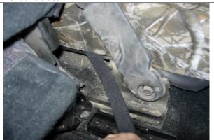
**Step 15. Middle Bottom/MB:** Route the side Velcro<sup>™</sup> at an angle to the carpet in back, and then tuck in the rear edge of the cover and pull back, connecting it to the carpet.
