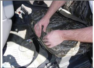
Step 9. Driver and Passenger Bottom/DB & PB: Work the material from the seam inside the seat cover from the inside to the outside edge (thumbs to fingers). Line up the seams of the seat cover to the seams of your seat, they should closely match. Mate the Velcro<sup>™</sup> behind where the seatbelt comes out of the seat bottom. Tuck in the back edge and pull it back but don't fasten it yet.
