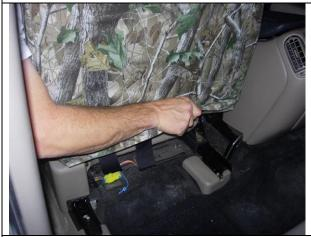
**Step 7. Driver and Passenger Tops/DT & PT:** Gently pull the Velcro<sup>™</sup> from behind the seat with one hand while using your other hand in a smoothing action in front of the seat from top to bottom. Tuck the Velcro<sup>™</sup> under the back edge and starting on the inside and work your way out.
