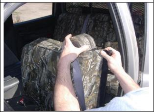
**Step 4. Driver & Passenger Tops/DT & PT:** Hold the top part in place with one hand and then connect the vertical Velcro<sup>™</sup> with the other.
