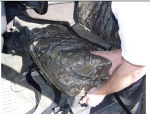
**Step 8. Driver and Passenger Bottom/DB & PB:** Place the seat cover bottoms on with the long hook (sticky) Velcro<sup>™</sup> to the front.
