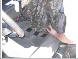
**Step 6. Driver & Passenger Tops/DT & PT:** Line up the seams of the seat cover to the seams of the seat, they should closely match. Next, tilt the backrest forward and tuck the extending hook (sticky) Velcro<sup>™</sup> into the seat.
