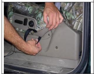
**Step 11. Driver and Passenger Bottom/DB & PB:** Slide the outside edge hook Velcro<sup>™</sup> up between the seat and the plastic. Carefully reach under the seat for the Velcro<sup>™</sup> and connect it at an angle to the carpet on the back edge.
