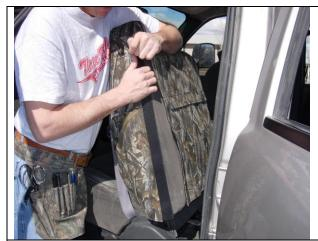
**Step 5. Driver & Passenger Tops/DT & PT:** Connect the vertical Velcro<sup>™</sup> by using a bear hug method starting at the top working your way down a few inches at a time.
