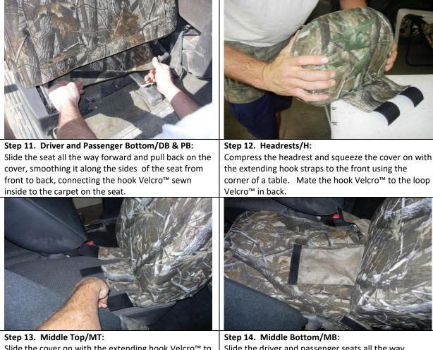
Slide the cover on with the extending hook Velcro<sup>M</sup> to the front, lining up the seams. Tuck the hook Velcro<sup>M</sup> in and mate them to the loop Velcro<sup>M</sup> inside the back edge.
