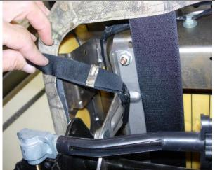
**Step 11. Driver and Passenger Bottom/DB & PB:** View from under the front of the driver's seat. Clip the plastic buckle over the metal as shown, then press the Velcro<sup>™</sup> together and trim the excess.
