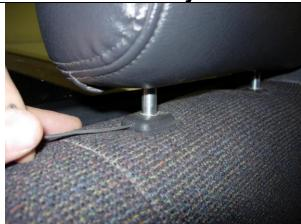
**Step 1. Driver & Passenger Tops/DT & PT** Temporarily remove the headrests by lifting it up all the way and inserting a heavy paper clip into the holes in the plastic as shown. Do this one at a time, gently lifting up and holding pressure until the headrest releases.
