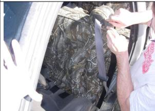
Step 3. Driver & Passenger Tops/DT & PT: Tuck the fabric under the plastic for the shoulder mounted seatbelt using a sawing motion to start, and then carefully use a thin metal object like a feeler gauge or a flat screwdriver to finish tucking the material.
