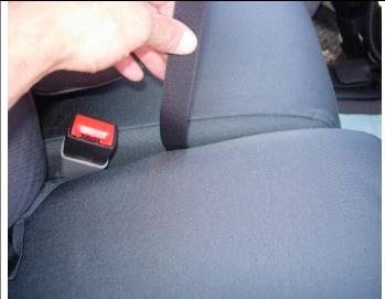
**Step 18. Driver and Passenger Bottoms:** View from behind the passenger seat. Pull the inside flap of the seat cover around to the back and connect it to the carpet on the back of the seat.
