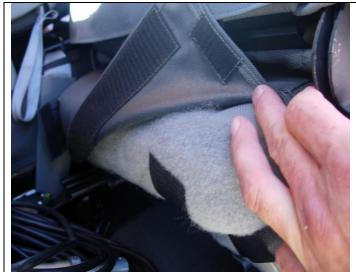
Step 17. Driver and Passenger Bottoms: Pull the rear edge of the seat cover back and lightly connect the hook Velcro<sup>™</sup> sewn on the inside to the carpet on the back edge of the seat, but not all the way. Make sure the position of the seat cover is correct by lining up the seams of the seat cover to the seams of your seats upholstery.
