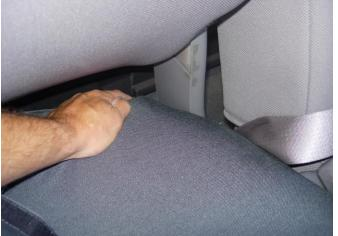
**Step 2. Middle Bottom/MB:** Fold the console part way down and tuck the left rear corner around the back of the seat.
