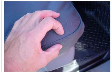
**Step 13. Driver and Passenger Bottoms:** Place the seat cover on with the long hook Velcro<sup>™</sup> to the front. Work the material from the seam inside the seat cover from inside (forefinger) to out (thumb). It takes a little doing, but this will produce a wrinkle free seam.
