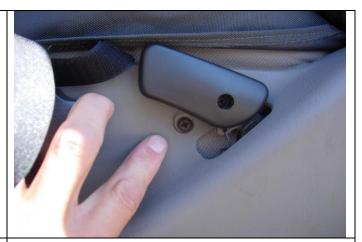
**Step 14. Driver and Passenger Bottoms:** Optional: Temporarily loosen the Phillips screw in the plastic below the recline lever. This will make the routing of the outside edge hook Velcro<sup>™</sup> between the seat and the plastic easier.
