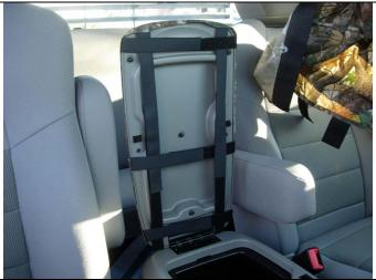
**Step 12. Lid/L:** Place the lid cover on by positioning the cut-out in front for the clipboard, then mating the Velcro<sup>™</sup> under the lid as shown. Some repositioning and tightening of the Velcro<sup>™</sup> may be needed to get it tight.
