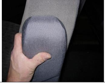
**Step 10. Driver & Passenger Armrests/DA&PA:** Work the top of the armrest cover down all the way. Fold the seams inside of the cover (where my forefinger is) to the middle (where my thumb is)
