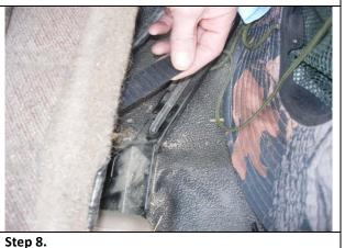
Pull it tight and mate it to the carpet on the back of the seat at roughly a 45 degree angle.
