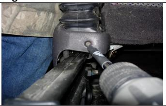
**Step 2. Driver and Passenger Bottoms:** Remove the screw from behind the seat as shown. The seat cover is labeled inside; refer to the "Seat Cover Piece Identification Chart" to identify the different pieces of the seat cover.
