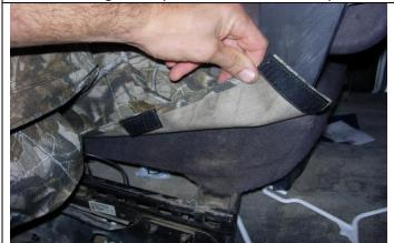
**Step 19. Middle Bottom:** Pull the left and right sides of the seat cover around to the back and connect the hook Velcro<sup>™</sup> to the carpet on the side and back of the seat. You may have to separate the front left and right hook Velcro<sup>™</sup> from the carpet and pull out slack
