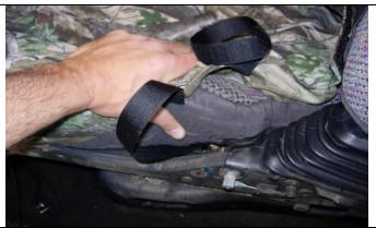
**Step 8. Driver and Passenger Bottoms:** Feed the long side hook Velcro<sup>™</sup> where shown and route to the back edge of the seat, connecting it to the carpet on the back edge of the seat. Route the inside Velcro<sup>™</sup> similarly to the carpet on the back of the seat.
