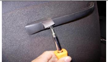
**Step 5 Driver and Passenger Tops/DT & PT:** Carefully pop this square rubber plug out using a flat screwdriver. Remove the screw using a # 25 Torx bit.
