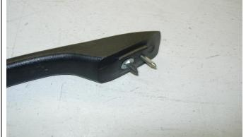
Step 6. Driver and Passenger Tops: Be sure to put the keeper washer back on the screw.
