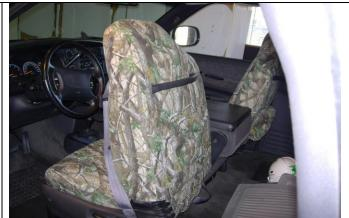
**Step 14. Driver and Passenger Tops:** Put the grab handle back on the seat, bolt the seatbelt back on and attach the plastic cowling.
