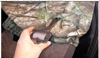
**Step 11. Driver and Passenger Tops:** Slide the seat cover on with the long hook Velcro<sup>™</sup> to the front. Feed the seat belt through the provided opening.
