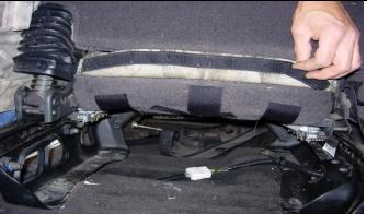
**Step 10. Driver and Passenger Bottoms:** Press the hook Velcro<sup>™</sup> sewn inside the back edge of the seat cover to the carpet on the back of the seat.
