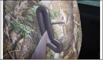
**Step 12. Driver and Passenger Tops:** Pull the cover down all the way on the left and right. Tuck the fabric behind the plastic for the seatbelt.
