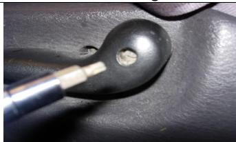
**Step 1. Driver and Passenger Bottoms/DB & PB:** Temporarily remove the outside edge plastic panel by removing the T-20 screws from the recline levers on the outsides of both seats. Next, Remove the Phillips screw shown behind the recline lever.
