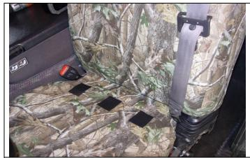
**Step 13. Driver and Passenger Tops:** Tuck the hook Velcro<sup>™</sup> into the seat and connect them to the loop Velcro<sup>™</sup> sewn inside the back edge.
