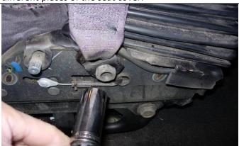
**Step 3. Driver and Passenger Bottoms:** Remove the screw in the front of the plastic panel.
