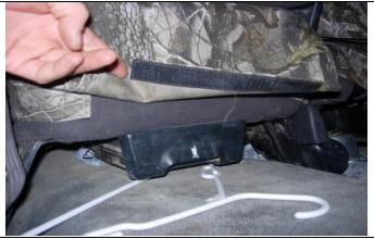
**Step 20. Middle Bottom:** Pull the seat cover back and connect the hook Velcro<sup>™</sup> sewn inside the back edge to the carpet on the seat above the plastic pull-out drink holders.
