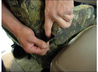
**Step 15. Driver and Passenger Armrests/DA&PA:** Connect the Velcro<sup>™</sup> at the back of the armrest covers as shown.
