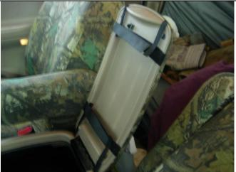
**Step 16. Lid/L:** Mate the fasteners under the lid as shown. Note: The lid cover was modified and looks different than the picture. The hook Velcro<sup>™</sup> in front extend and connect to the rear Velcro<sup>™</sup>.
