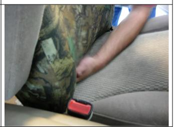
**Step 4. Driver and Passenger Tops/DT&PT:** Tuck the hook Velcro<sup>™</sup> into the seat and connect them to the loop Velcro<sup>™</sup> sewn in back. Do this by using one hand in a smoothing action down the front of the seat from top to bottom while gently pulling on the front hook Velcro<sup>™</sup>, and then tuck it under the back edge and pressing them together.
