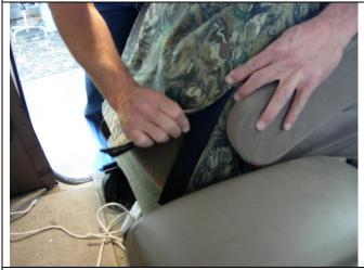
**Step 3. Driver and Passenger Tops/DT&PT:** Connect the Velcro<sup>™</sup> under the armrest starting under the armrest and work your way down as shown.
