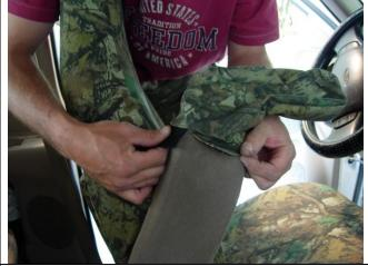
**Step 13. Driver and Passenger Armrests/DA&PA:** Slide the cover on with the cut out towards the seat.
