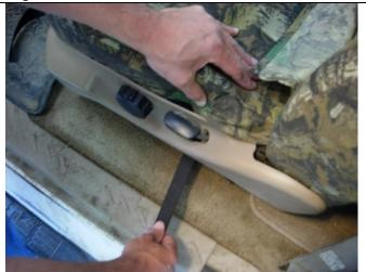
**Step 8. Driver and Passenger Bottoms/DB&PB:** Pull the Velcro<sup>™</sup> through to the bottom of the plastic and tuck the fabric behind the plastic cowling.
