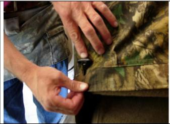
**Step 2. Driver and Passenger Tops/DT&PT:** Work the access lever through the provided opening behind the seat. Line up the seams of the seat cover to the seams of your seat, they should closely match.
