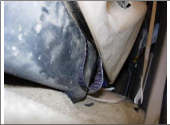
**Step 9. Driver and Passenger Bottoms/DB&PB:** Route the outside edge hook Velcro<sup>™</sup> between the seat slide and the seat as shown and press it to the carpet on the back edge of the seat.
