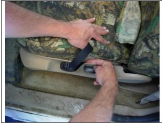
**Step 7. Driver and Passenger Bottoms/DB&PB:** Slide the long outside edge hook Velcro<sup>™</sup> between the seat and the plastic. Route the Velcro<sup>™</sup> between the recline lever and the lumbar knob.
