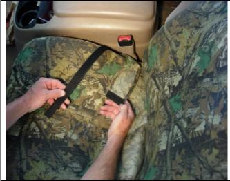
**Step 5. Driver and Passenger Bottoms/DB&PB:** Place the seat covers on with the long hook Velcro<sup>™</sup> to the front and the long flap of material (shown in right hand) to the inside.
