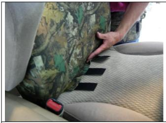
**Step 1. Driver and Passenger Tops/DT&PT:** The parts of the seat covers are labeled inside. Use the "Seat Cover Piece Identification Chart" to identify the parts. Slide the seat cover on with the long hook Velcro<sup>™</sup> (sticky) to the front and the cut-out for the armrest to the inside.
