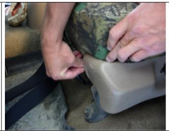
**Step 6. Driver and Passenger Bottoms/DB&PB:** Tuck the material of the seat cover behind the plastic cowling in front. Route the long hook Velcro<sup>™</sup> under the seat and press them to the carpet on the back edge of the seat.
