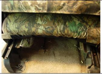
**Step 10. Driver and Passenger Bottoms/DB&PB:** Pull the inside of the edge of the seat around to the back of the seat and mate it to the carpet on the back edge of the seat. The flap is on the right side of the photo. Route the long inside hook Velcro<sup>™</sup> around the back inside corner of the seat, mating it to the carpet.
