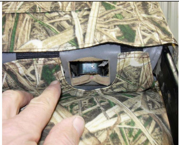
Step 18. Driver & Passenger Top/DT&PT: Use one hand in a smoothing action down the front of the seat cover while gently pulling on the Velcro from behind, then connect the Velcro™.
