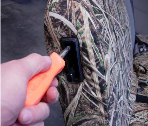
Step 15. Driver & Passenger Top/DT&PT: Tighten the screws for the side latch.
