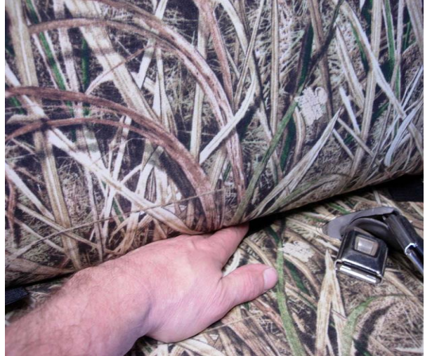
Step 16. Driver & Passenger Top/DT&PT: Tuck in the front of the seat cover and fold the backrest forward.
