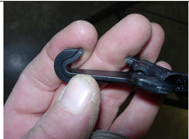
Step 8. Bottom/B: Next, clip off the front of the hook as shown.
