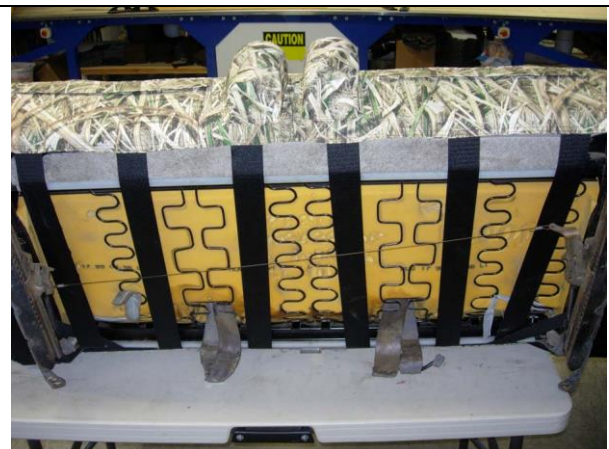
Step 10. Bottom/B: Route the long hook Velcro™ under the seat to the back edge, making sure to route them between the seat and the seat slide wire as to not impede it.
