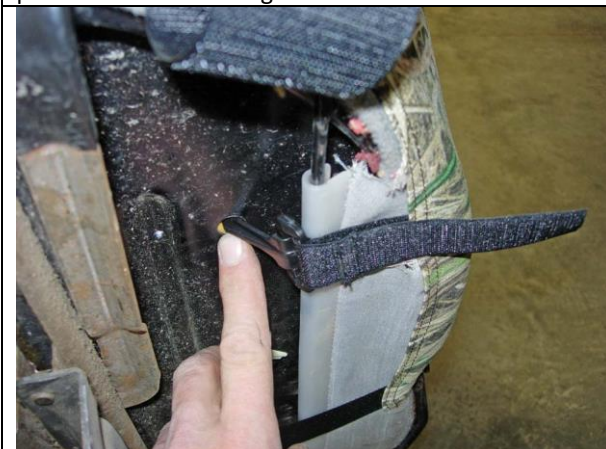
Step 9. Bottom/B: Push the hook into the hole in the metal pan under the outside edge, then connect the Velcro™, trimming the excess.
