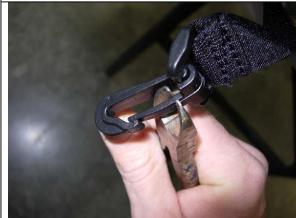
Step 7. Bottom/B: Using a side cutter, clip off the safety catch from the plastic buckle on the right and left.
