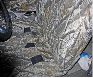
Step 2. Driver and Passenger Tops/DT & PT: Slide the seat cover on with the extending hook Velcro™ to the front.
