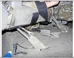
Step 9. Driver and Passenger Bottoms/DB & PB: Tuck in the rear most part of the seat cover, pull it back hard and press the Velcro™ to the carpet on the back edge of the seat.
