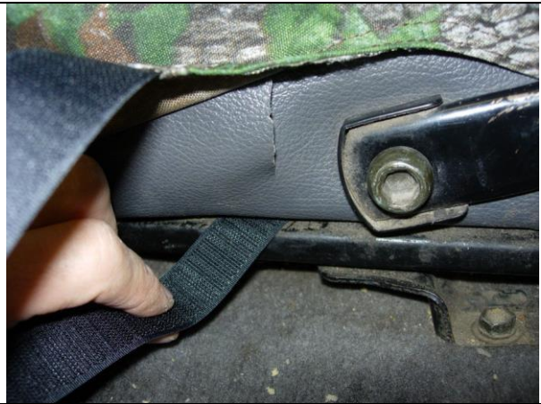
Step 8. Bottom/B Route the hook Velcro™ between the seat slide and the seat, just in front of the hinge arm.
