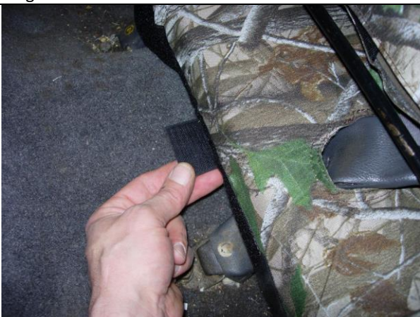
Step 11. Bottom/B Slide the seat all the way forward and route the long front hook Velcro™ under the seat. Mate them to the loop Velcro™ on back. The two center Velcro™ route easiest along the transmission hump.
