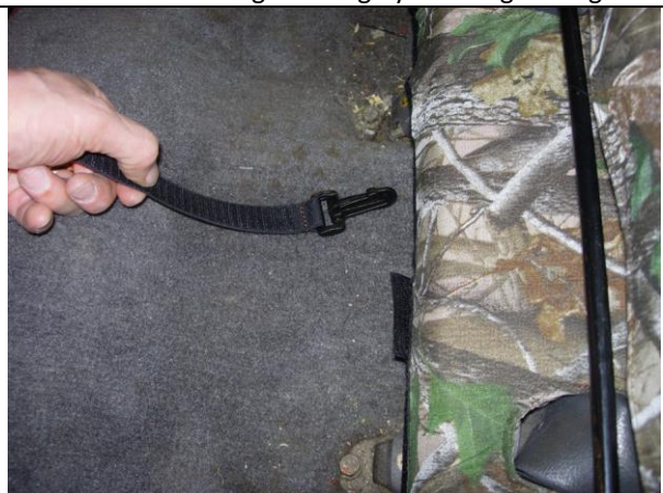
Step 12. Bottom/B Connect the three plastic buckles under the back edge of the seat. One in the middle, one for passenger, and one for the driver side. See step 15 for view.
