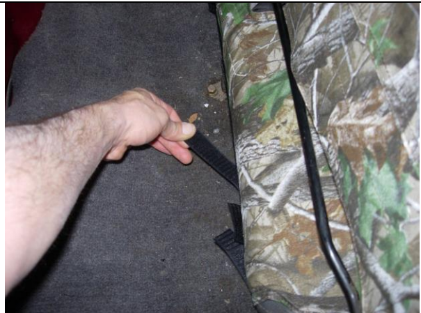
Step 10. Bottom/B Mate both side hook Velcro™ to the loop Velcro™ sewn on the back edge at roughly a 45 degree angle.
