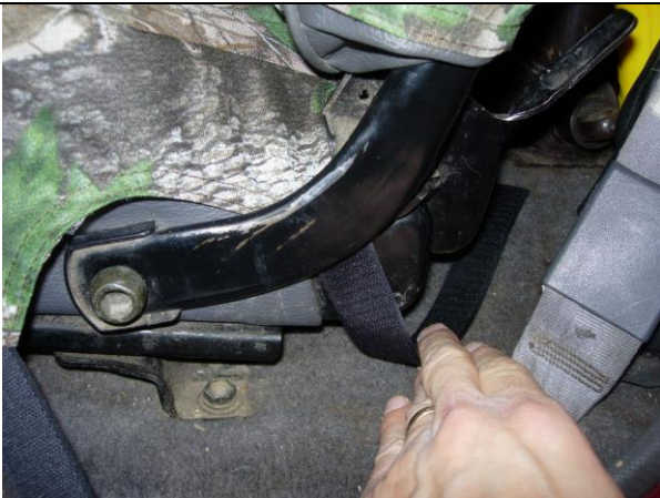
Step 9. Bottom/B Route the rear most side hook Velcro™ behind the hinge arm and route it around the back corner.
