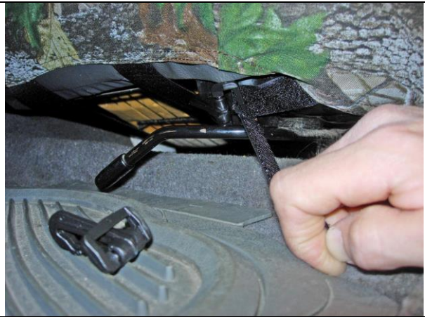
Step 16. Bottom/B Fasten the side buckle to the 3" wide metal frame, then back to itself. Trim excess if necessary.
