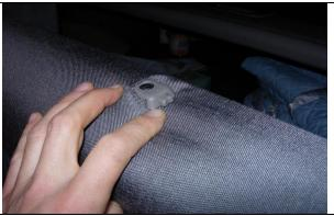
**Step 2. Driver & Passenger Tops/DT&PT:** Side the seat covers on with the labels DT & PT to the front. Tuck the fabric of the seat cover under the plastic for the headrest. Line up the seams of the seat cover to the seams of your seat, they should closely match.
