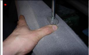
**Step 1. Driver & Passenger Tops/DT&PT:** All the parts of your seat cover are labeled inside. Use the "Seat Cover Piece Identification Chart" to ID parts. Temporarily remove the headrests by depressing the push button release and lifting up.
