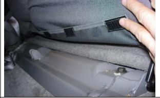
**Step 6. Driver & Passenger Tops/DT&PT:** Press the front edge of the seat cover to the fuzzy carpet working from one side to the other.
