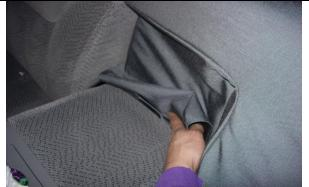
**Step 3. Driver Top/DT:** Tuck the fabric in behind the hinge next the armrest.
