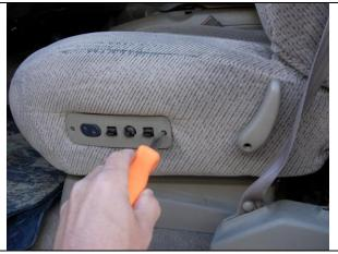
**Step 5. Driver and Passenger Bottoms/DB & PB:** Loosen the screws on the plastic seat control panels and remove the recline levers using a Phillips screwdriver.
