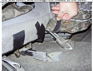
Step 7. Driver and Passenger Bottoms/DB & PB: View from behind the driver's seat. Pull the inside edge of the seat cover around to the back and press the hook Velcro™ to the carpet on the back of the seat
