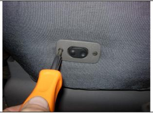
**Step 5. Driver and Passenger Bottoms/DB & PB:** Loosen the screws from the plastic seat control panels and remove the recline and access levers using a Phillips screwdriver.
