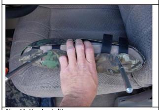
**Step 11. Headrests/H:**Tuck them under the back edge and connect them to the loop Velcro™ sewn inside the back edge.
