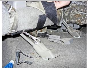
**Step 9. Driver and Passenger Bottoms/DB & PB:** Tuck in the rear most part of the seat cover, pull back hard and press it to the carpet on the back edge of the seat.
