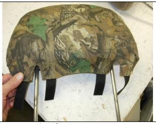
Step 10. Headrests/H: Slide the cover on with the extending hook  $Velcro^{TM}$  to the front.
