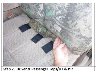
Tuck the hook Velcro™ into the seat, slide the seat all the way forward tipping the backrest ahead.
