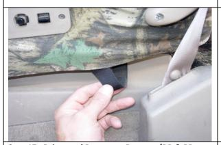
Step 17. Driver and Passenger Bottoms/DB & PB: Route the long side hook Velcro™ under the seat, avoiding the mechanisms, at an angle to the back edge to the seat. NOTE: The passenger side doesn't have an
