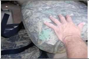
**Step 15. Driver and Passenger Bottoms/DB & PB:** Pull on the back edge of the cover and make sure it's all the way back and snug to the front of the seat.
