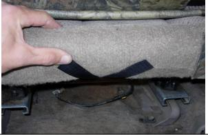
Step 18. Driver and Passenger Bottoms/DB & PB: press the long side hook Velcro™ in a crossing fashion forming an "X" on the carpet on the back edge of the seat
