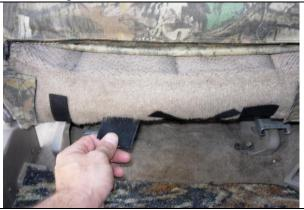
Step 21. Driver and Passenger Bottoms/DB & PB: Pull the long hook Velcro™ back and press them to the carpet as shown.
