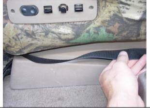
Step 19. Driver and Passenger Bottoms/DB & PB: Route the 1" wide long front hook Velcro™ along the outside edge of the seat and press it to the carpet on the back edge of the seat.
