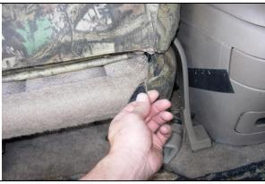
**Step 16. Driver and Passenger Bottoms/DB & PB:** Pull the inside edge (next to the console) of the cover back and press it to the carpet on the back of the seat. Next, do the same for the outside edge of the cover.
