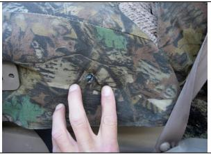
**Step 14. Driver and Passenger Bottoms/DB & PB:** Locate the hole provided for the recline lever, feeding the post for the lever through the hole. Install the recline lever onto the seat.
